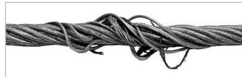
Loops have formed in the wire rope.
