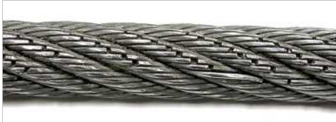
Multiple broken wires. Broken wires are signs of normal wear of the wire rope. They occur when the wire rope is bent on the reels under load.
