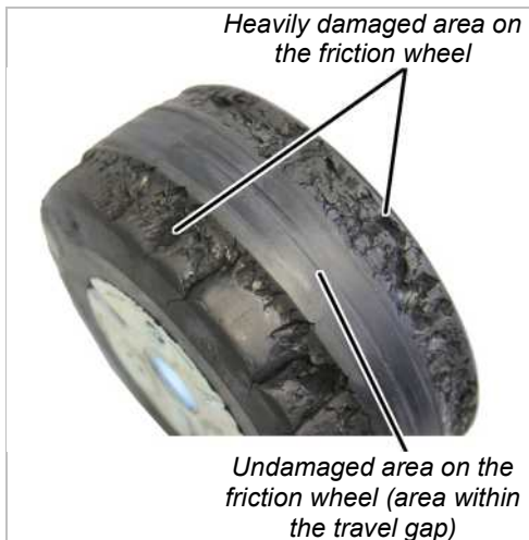
Example of damage on the friction wheel.
